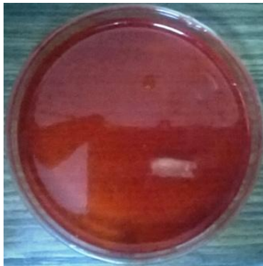
Figure 3: Zymogram analysis, on plate (stained with congo red) showing zones of clearance around bands corresponding to partially purified chitinase enzyme
