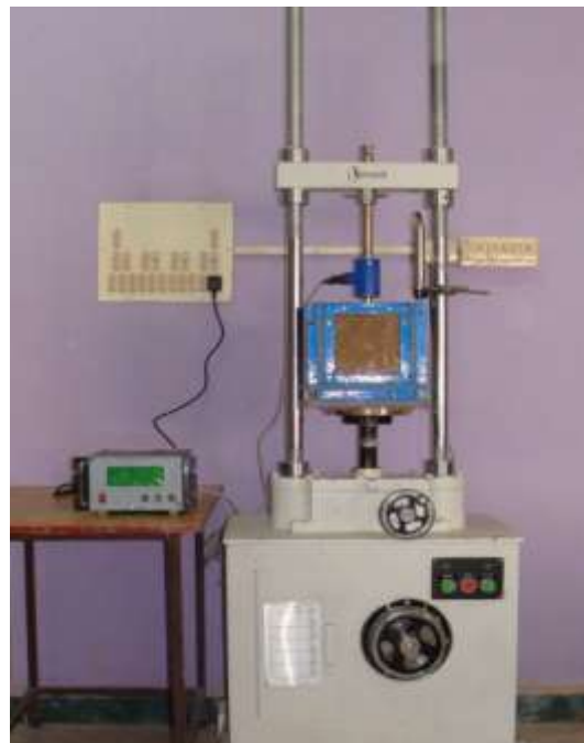
Fig 5. Experimental set up for testing the soil specimen
